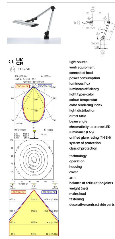
LED electronic ballast 100-240 V, 50/60 Hz; secondary 24 V, DC env. 23 W approx. 1.500 lm approx. 78 lm/W cold white approx. 5.000 K CRI > 90; R9 > 50 direct approx. 100 % 75° < 3 SDCM <= 12000 cd/m<sup>2</sup> <= 25 IP 20 I with plug-in power supply; III without plug-in power supply Touch DIM multi-function switch aluminium coloured anodised structured; plastic silver metallic spring ca. 1,9 kg ca. 3,4 m; mains plug; CEE 7/VII table base black
